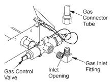
Figure 10 - Installing Inlet Fitting and Gas Connector Tube
